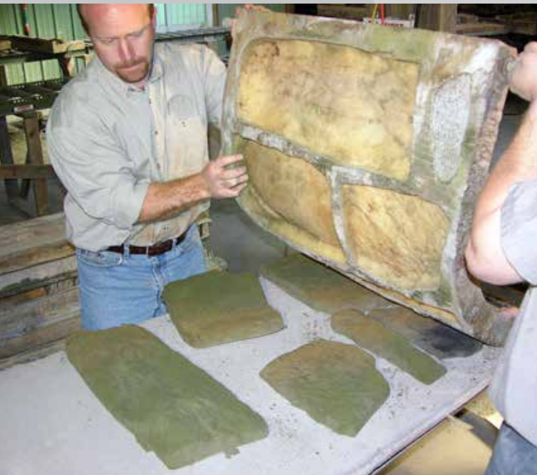
5 Cast stones are demolded and inspected to ensure quality.
