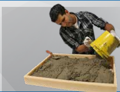
6 CONCRETE IS POURED INTO PREPARED MOLD OF PLAQUE
