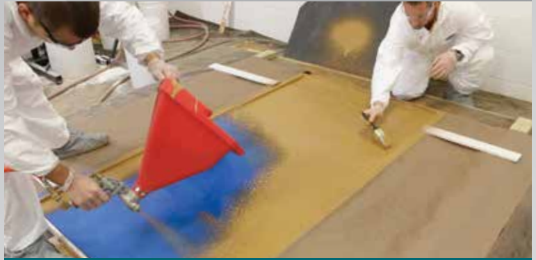
6 A hopper gun is used to spray the GFRC face coat.
