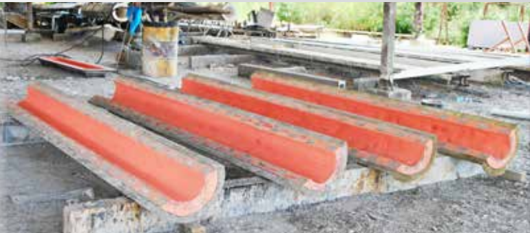
9 Rebound™ 25 was also used to capture intricate detail from the bark of a Banyan tree. Molds were used to make GFRG posts used to support the GFRG wall segments.
