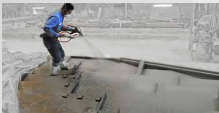
2 Additional layers of backup mix reinforced with AR glass fiber are applied.
