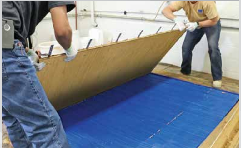
8 Four GFRC panels of different sizes will be made from the same mold
