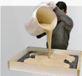
3 VYTALEX™ MOLD RUBBER IS POURED
