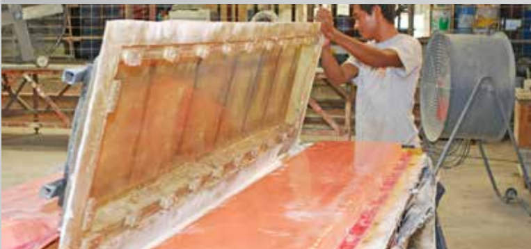
5 The support shell is separated from the rubber mold. The mold can then be removed from the original bamboo model.
