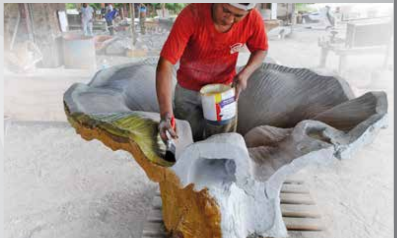
8 A multi-step staining process makes the GFRC casting look exactly like the original.
