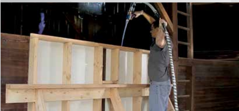
2 Mold Star™ 30 is dispensed, quickly filling the gap.
