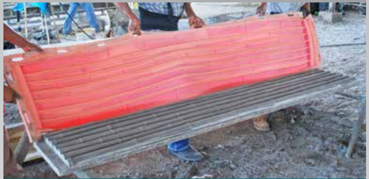
8 The GFRG panel reflects all of the detail of the original bamboo model. The concrete pieces can be stained for a realistic finish.
