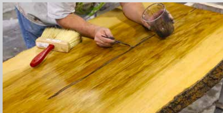
6 Soft brushes are used to feather the Buddy Rhodes Glazes to simulate natural wood grain.
