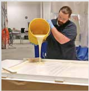
3 VytaFlex™ 60 is properly measured, mixed and poured over the entire model.
