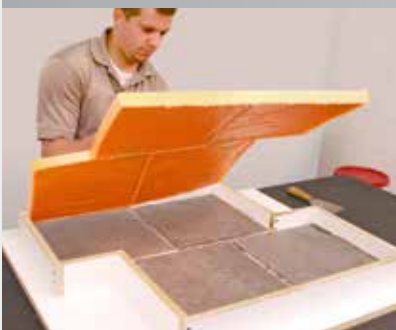
5 Once cured, stamp is demolded. Multiple stamps are made for a single job.
