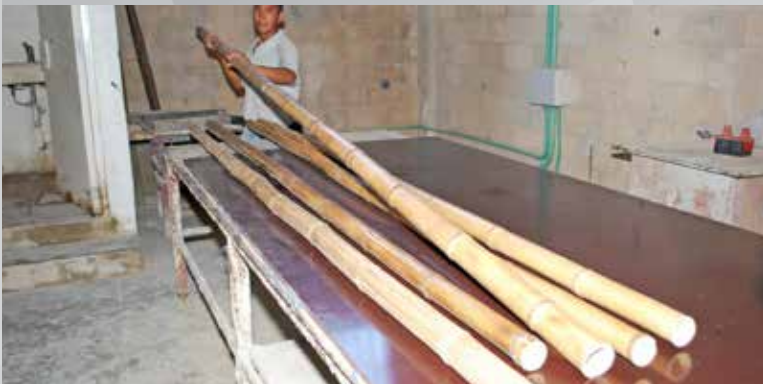
1 To create the original pattern, similar size pieces of bamboo were selected and cut in half.
