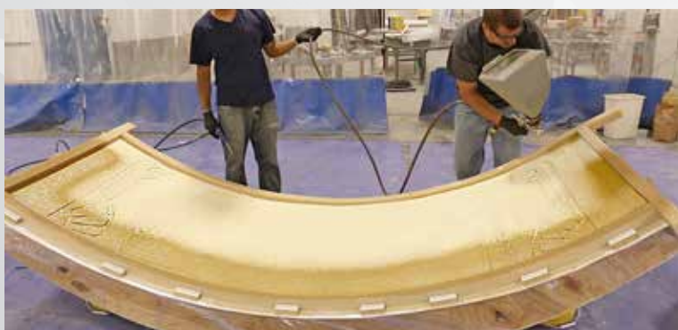
5 The GFRc face mix is sprayed using a hopper gun.
