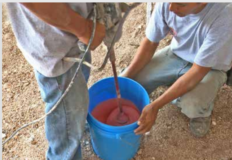
2 Rebound™ 25 mold rubber is dispensed 1A:1B by volume. A drill mixer is used to thoroughly mix the two parts.
