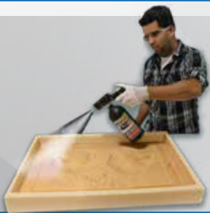
5 AQUACON™ IS APPLIED TO THE MOLD WITH THE KWIKIEE™ SPRAYER
