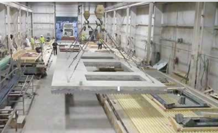
7 An overhead crane is used to lift and demold the 41,000 lb (18,600 kgs) concrete panel.
