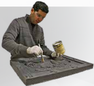
1 SONITE™ WAX IS APPLIED TO SEAL THE ORIGINAL MODEL
