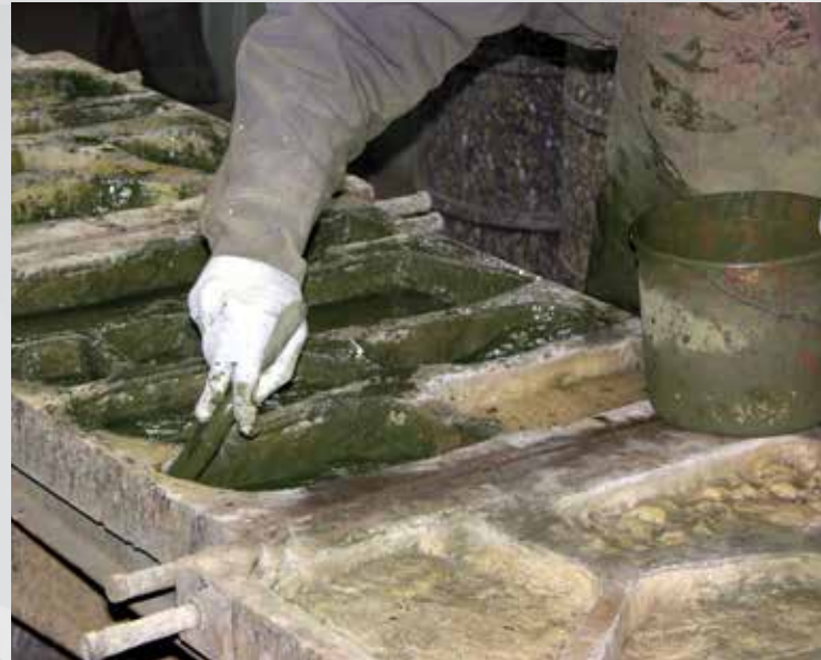
2 Mold cavity is pigmented to desired color.
