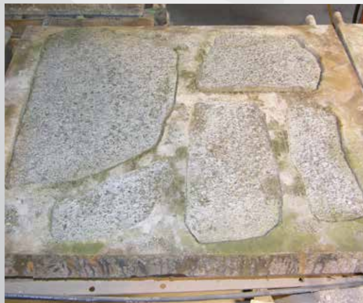
4 Concrete is allowed to set fully.
