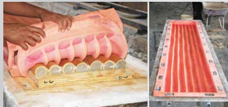
6 The Rebound™ mold reflects perfect detail captured from the bamboo. The rubber mold is seated into the support shell and is ready for casting.
