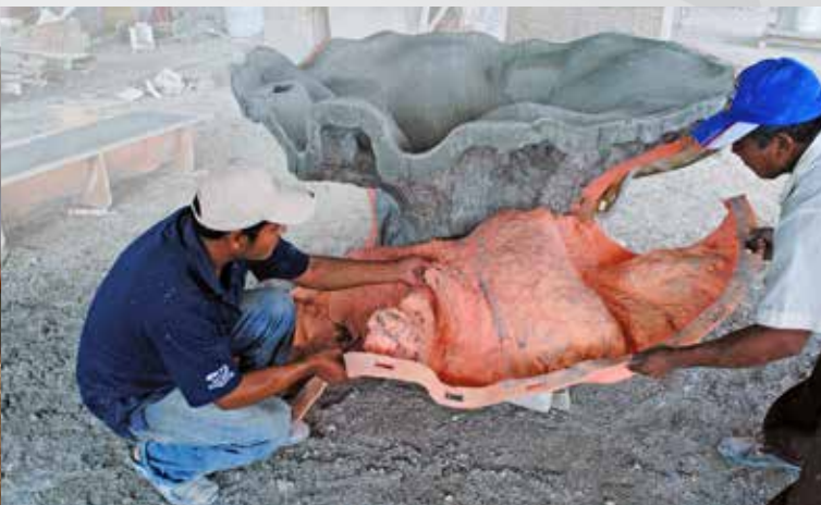
7 Finished GFRC casting is removed from the Rebound™ 25 rubber mold.
